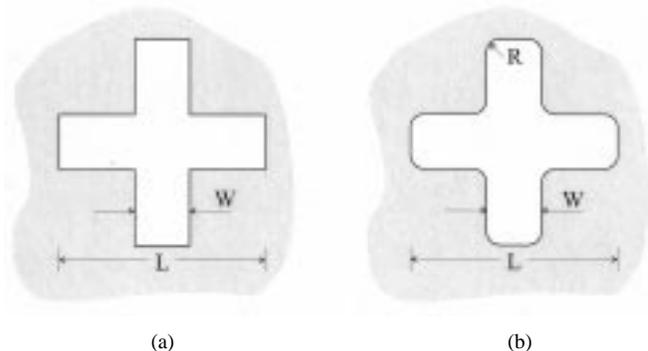
Fig. 9. Geometry of the aperture of the quasi-optical filter: (a) the cross with sharp corners and (b) the cross with rounded corners. The dimensions of the aperture and the periodicity are:  $L = 570 \mu\text{m}$ ,  $W = 160 \mu\text{m}$ ,  $R = 40 \mu\text{m}$ ,  $a = b = 810 \mu\text{m}$ , and  $\alpha = 90^\circ$ .
