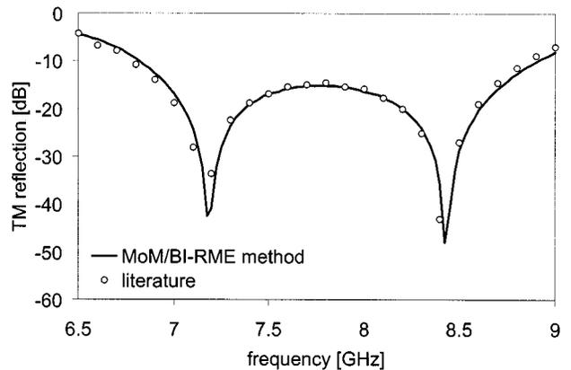
Fig. 6. Analysis of the  $X$ -band dichroic filter with infinitely thin metal walls ( $w = 0$ ): MoM/BI-RME analysis is compared with simulations reported in the literature.
