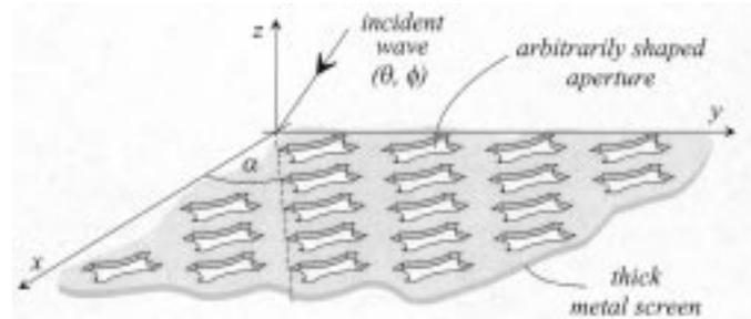
Fig. 1. A quasi-optical filter with arbitrarily shaped apertures.
