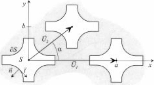
Fig. 2. Periodicity of the quasi-optical structure:  $\vec{U}_1 = a\vec{u}_x$ ,  $\vec{U}_2 = b/\tan\alpha\vec{u}_x + b\vec{u}_y$ .
