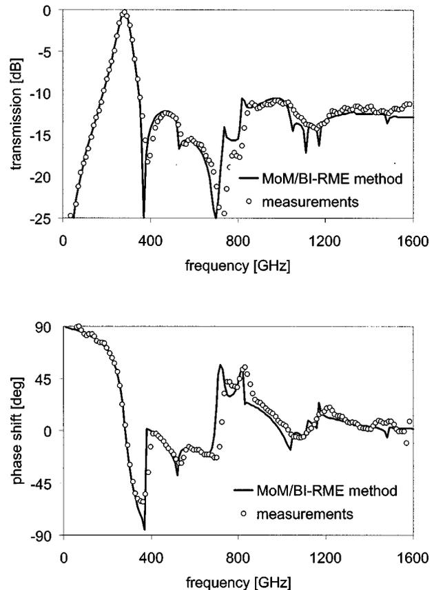
Fig. 11. Numerical results for the filter considering the aperture shape with rounded corners [Fig. 9(b)], compared with experimental data.
