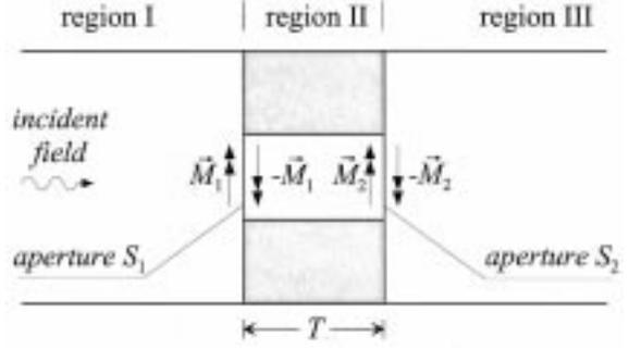
Fig. 3. Side view of the equivalent circuit of the unit cell. Region II is a waveguide section with a cross section  $S$ , connected to Regions I and III through the apertures  $S_1$  and  $S_2$ , respectively.
