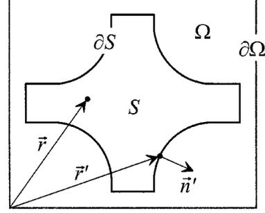
Fig. 4. The geometry considered for the application of the BI-RME method: the cross section  $S$  of the arbitrarily shaped waveguide is enclosed in the exterior rectangular resonator  $\Omega$ .
