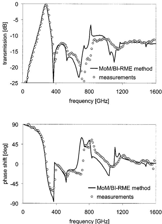
Fig. 10. Numerical results for the filter considering the aperture shape with sharp corners [Fig. 9(a)], compared with experimental data. The transmittance phase is the difference between the phase measured with and without the filter.
