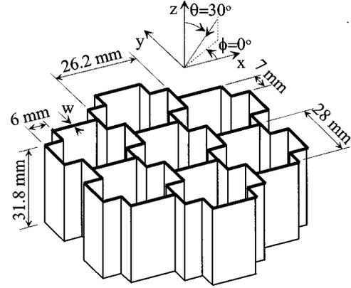
Fig. 5. Schematic representation of the  $X$ -band dichroic filter. In the prototype, the wall thickness was  $w = 0.41$  mm. The angle of incidence is  $\theta = 30^\circ, \phi = 0^\circ$ .
