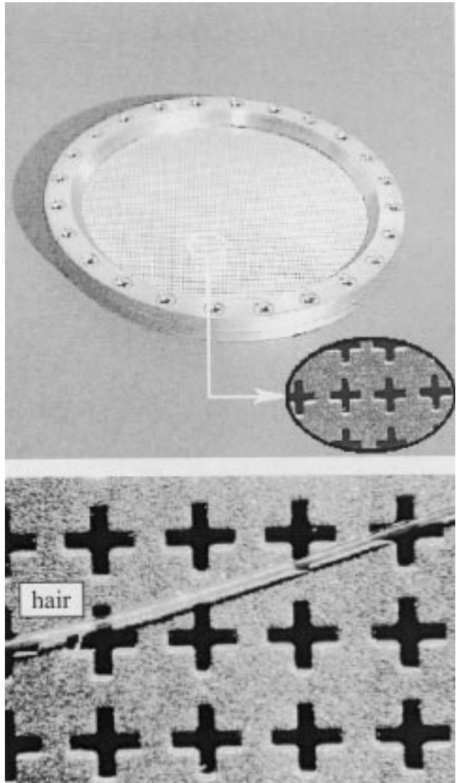
Fig. 8. Photographs of the 280-GHz quasi-optical filter.
