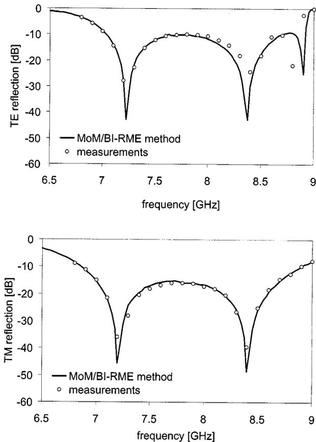
Fig. 7. Analysis of the X-band dichroic filter with metal walls of finite thickness ( $w = 0.41$  mm): MoM/BI-RME analysis is compared with measurements reported in the literature.
