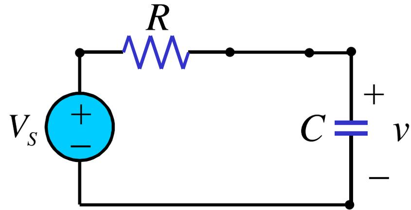
$$\frac{d(v - V_S)}{dt} + \frac{v - V_S}{RC} = 0 \quad \Rightarrow \quad v(t) - V_S = Ae^{-t/RC} \quad \Leftarrow \quad v(0^+) = V_0$$
