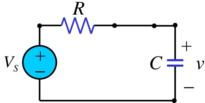
$$\frac{d(v - V_S)}{dt} + \frac{v - V_S}{RC} = 0 \quad \Rightarrow \quad v(t) - V_S = Ae^{-t/RC} \quad \Leftarrow \quad v(0^+) = V_0$$
