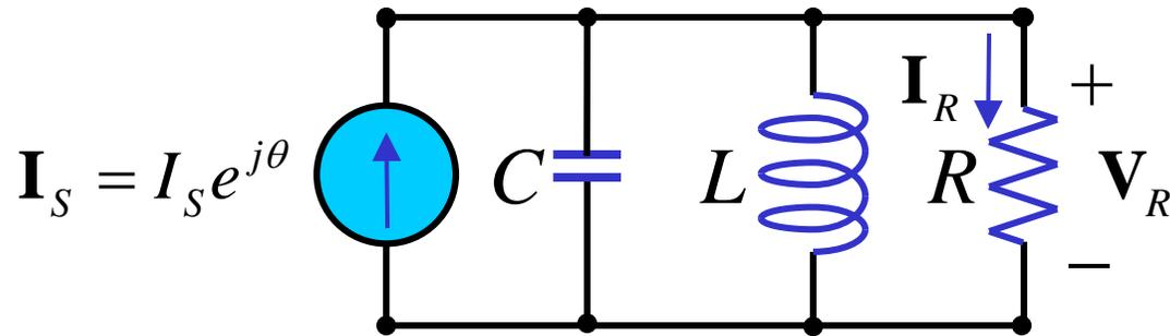
$$\mathbf{H}(\omega) = H(\omega)e^{j\phi(\omega)} = \frac{\mathbf{I}_R}{\mathbf{I}_s} = \frac{1/R}{1/R + j\omega C + 1/j\omega L} = \frac{1}{1 + j\left(\omega RC - \frac{R}{\omega L}\right)}$$
