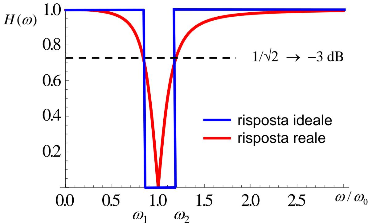
$$\mathbf{H}(\omega) = \frac{\mathbf{V}_{LC}}{\mathbf{V}_S} = \frac{jQ \left( \frac{\omega}{\omega_0} - \frac{\omega_0}{\omega} \right)}{1 + jQ \left( \frac{\omega}{\omega_0} - \frac{\omega_0}{\omega} \right)}$$
