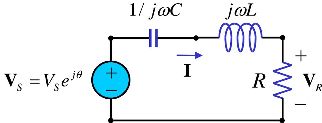
$$\mathbf{H}(\omega) = H(\omega)e^{j\phi(\omega)} = \frac{\mathbf{V}_R}{\mathbf{V}_S} = \frac{R}{R + 1/j\omega C + j\omega L} = \frac{1}{1 + j\left(\frac{\omega L}{R} - \frac{1}{\omega RC}\right)}$$
