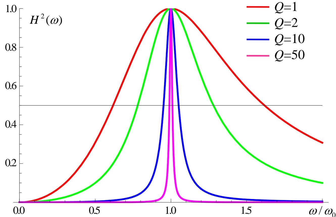
$$H^2(\omega) = \frac{1}{1 + Q^2 \left( \frac{\omega}{\omega_0} - \frac{\omega_0}{\omega} \right)^2}$$
