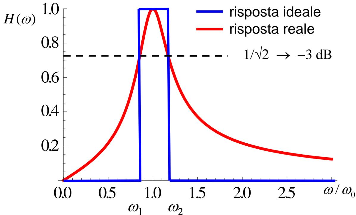
$$\mathbf{H}(\omega) = \frac{\mathbf{V}_R}{\mathbf{V}_S} = \frac{1}{1 + jQ \left( \frac{\omega}{\omega_0} - \frac{\omega_0}{\omega} \right)}$$
