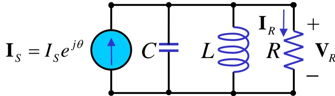
$$H(\omega) = \frac{1}{\sqrt{1 + \left( \omega RC - \frac{R}{\omega L} \right)^2}}$$
